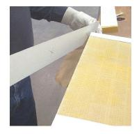
Immediately trim using knife as shown. Cut against a hard surface. Note that cutting short ends first helps prevent tearing the mat.
